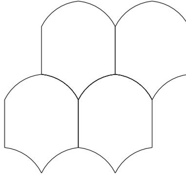
Figure 3. Example of a periodic foam ‘loaded’ by the weight of its Plateau borders. In this two-dimensional example, the Plateau borders are the isolated triple junctions, where three bubbles meet. The piece of the foam shown repeats by translation, and there is a vertical pressure gradient.
